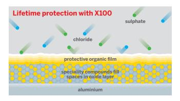
X100 contains 5 specialist inhibitors for unrivalled protection of aluminium. The speciality corrosion inhibitors create a denser, less penetrable layer which is topped off with a protective organic film, to completely protect aluminium from the damaging effects of corrosion.
