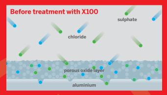
If left untreated, system metals such as aluminium and stainless steel are open to attack in water by aggressive chloride and sulphate compounds. Natural oxide layers are easily penetrated, which quickly leads to pitting and corrosion, putting high value components at risk of damage or failure.
