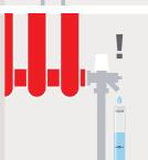
**3:** If the circles are visible above line A the system is clean but may require topping up with X100 Inhibitor to maintain system protection.
