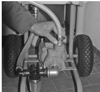
1. Connect pressure hose to pump outlet
