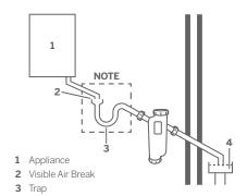
Open end of condensate drainage pipe direct into gully below grating but above water level
